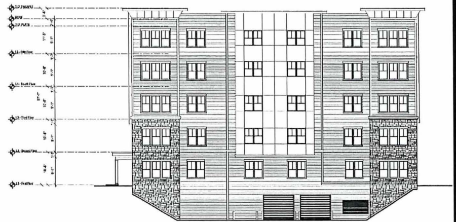
② RIGHT SIDE ELEVATION 1/8" = 1' 0"
