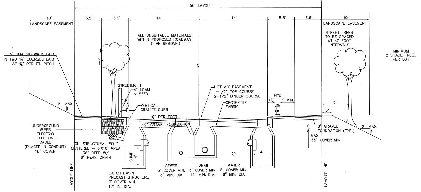
MAINTAIN 10' MIN. HORIZONTAL SEPARATION BETWEEN SEWER & WATER MAINTAIN 5' MIN. HORIZONTAL SEPARATION BETWEEN ALL OTHER UTILITY PIPES MAINTAIN 5' MIN. HORIZONTAL SEPARATION BETWEEN ALL UTILITY STRUCTURES MAINTAIN 1' MIN. VERTICALL SEPARATION BETWEEN ALL UTILITIES
