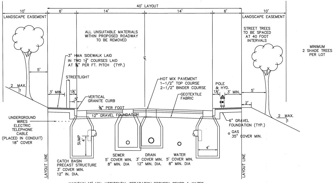
MAINTAIN 10' MIN. HORIZONTAL SEPARATION BETWEEN SEWER & WATER MAINTAIN 5' MIN. HORIZONTAL SEPARATION BETWEEN ALL OTHER UTILITY PIPES MAINTAIN 5' MIN. HORIZONTAL SEPARATION BETWEEN ALL UTILITY STRUCTURES MAINTAIN 1' MIN. VERTICALL SEPARATION BETWEEN ALL UTILITIES
