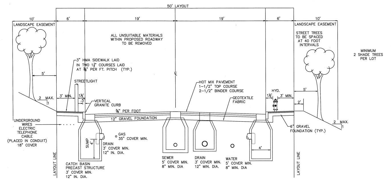
MAINTAIN 10' MIN. HORIZONTAL SEPARATION BETWEEN SEWER & WATER MAINTAIN 5' MIN. HORIZONTAL SEPARATION BETWEEN ALL OTHER UTILITY PIPES MAINTAIN 5' MIN. HORIZONTAL SEPARATION BETWEEN ALL UTILITY STRUCTURES MAINTAIN 1' MIN. VERTICALL SEPARATION BETWEEN ALL UTILITIES
